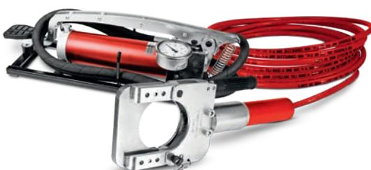
Safety hydraulic cable cutting set for Al and Cu cables, when the voltage is impossible to determine. Equipped with hydraulic head, pump with manometer and automatic retraction, earthing wire, hydraulic hose (10 m). Maximum nominal tension – 60 kV.
