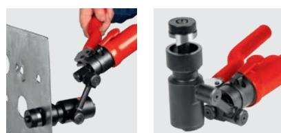
Hydraulic punching tool for punching round, square and rectangular holes.
