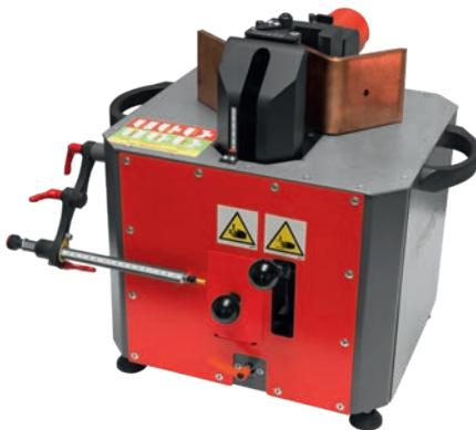
Station for cutting, hole punching, bending and offsetting Al and Cu busbars as well as inserting nuts:
