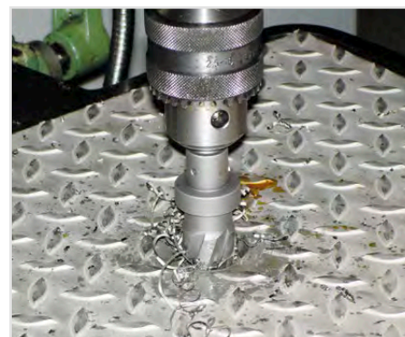
Drilling structured sheet metals
