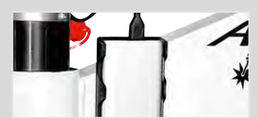
Laser pointer for optical display of tool centre and power bank
