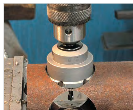
Drilling in pipes
