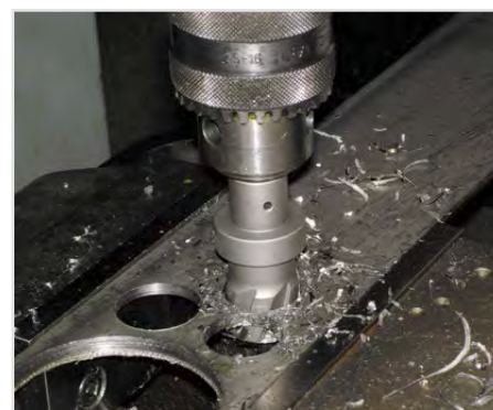
Drilling flat steels
