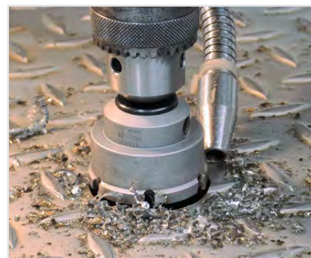
Drilling in checker sheet
