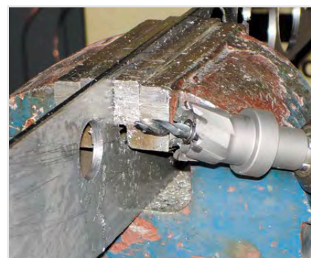
Free-hand drilling up to Ø 30 mm
