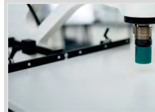
Length and depth limit stop with foldable add-on stops
