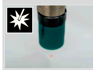
Laser pointer for optical display of tool centre and power bank
