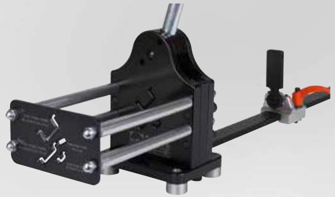
Guidance fixture for 90° angle-precise cutting
