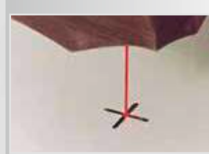
Laser pointer for optical display of tool centre
