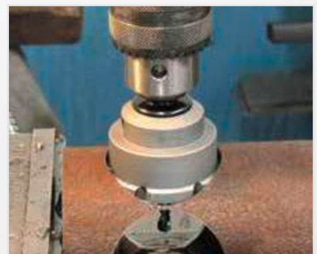
Drilling in pipes
