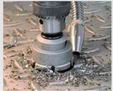
Drilling in checker sheet
