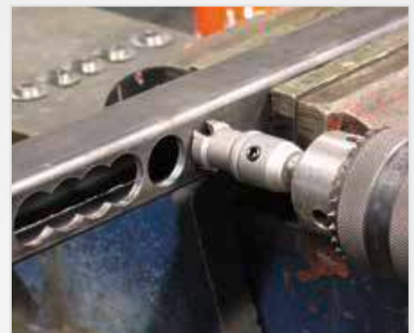
Drilling in square profiles
