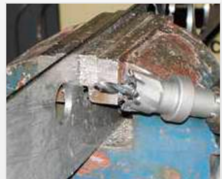
Free-hand drilling up to Ø 30 mm
