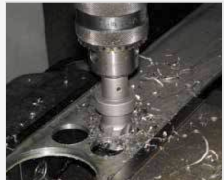
Drilling flat steels
